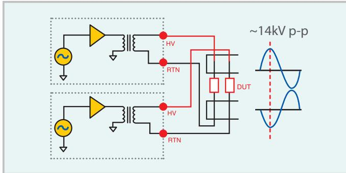
Figure 1 : Unsynchronized Output
