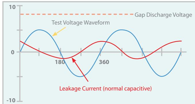
Figure 3 : Normal Leakage Current Waveform
