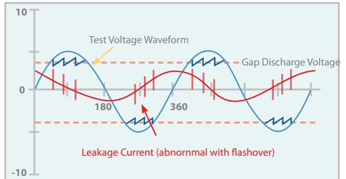
Figure 4 : Leakage Current Waveform when Flashover occurred
